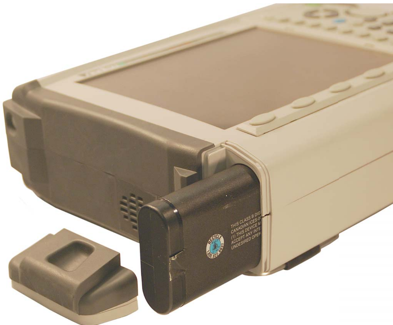
Figure 5-5. MS2026C/MS2027C/MS2028C/MS2036C/MS2037C/MS2038C Case, Battery Door, and Battery
